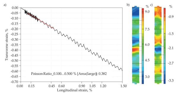
Fig. 5. Determination of Poisson's ratio: a) strain diagram, b) distribution of axial strains  $\varepsilon_{y}$ , c) distribution of transverse strains  $\varepsilon_{z}$
