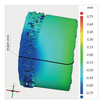
Fig. 8. Presentation of the results of flexspline deformation measurement in GOM
