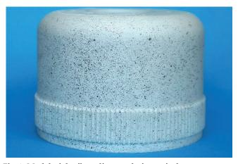
Fig. 3. Model of the flexspline, ready for optical measurements
