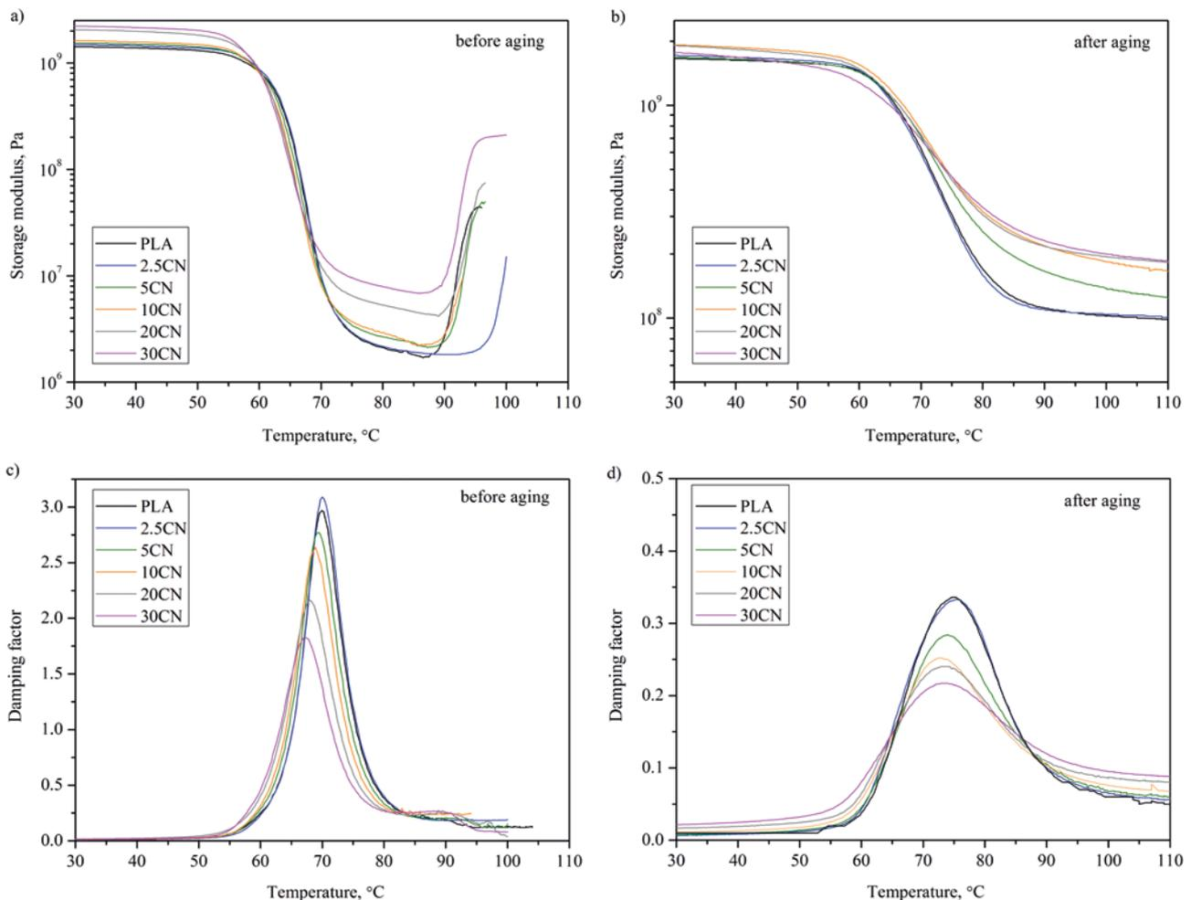
Fig. 4. a, b) Storage modulus ( $G'$ ), c, d) damping factor ( $\tan \delta$ ) of PLA and PLA composites before (a, c) and after (b, d) aging process
