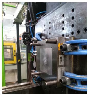
Fig. 6. Injection mold seat for the KZ25 gear wheel
