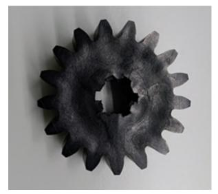
Fig. 8. Defects of KZ25 (P6) moldings: a) burns on the connection lines and tooth tips, b) collapsed
