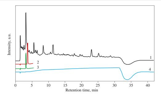
*Fig.* 1. HPAEC chromatograms of chitosan oligomers (1), glucosamine (2), and acetylglucosamine (3) in comparison with basic line (4)
