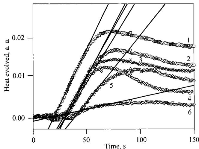
Fig. 7. The family of kinetic curves recorded during an argon-ion laser initiated polymerization of TMPTA in the presence of: 1 — Rose bengal C2' propyl ester ( $c = 2 \cdot 10^{-4}$  M) and ethyl 4-*N,N*-(dimethylamino)benzoate ( $c = 10^{-3}$  M), 2 — DDRB ( $c = 10^{-3}$  M), 3 — HDRB ( $c = 10^{-3}$  M), 4 — BDRB ( $c = 10^{-3}$  M), 5 — PDRB ( $c = 10^{-3}$  M), 6 — XDRB ( $c = 10^{-3}$  M)
