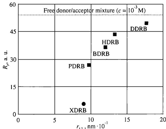
Fig. 8. Relationship between the rate of polymerization ( $R_p$ ) and the distance separating the donor and acceptor moieties ( $r_{12}$ ) (calculated for stress-free molecules using AM1 method) for tested A-S-D photoinitiators
