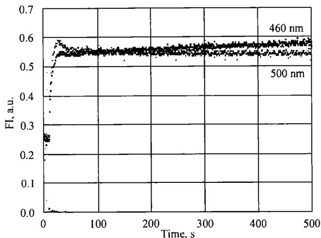
Fig. 4. The change of densylamide fluorescence intensity (FI) recorded during the irradiation of TMPTMA/VP (9:1) mixture; photoinitiation system: Poly-RB-OAc ( $5 \cdot 10^{-4}$  M of RB-OAc molecules), NPG (0.05 M); mode of irradiation — see Fig. 1
