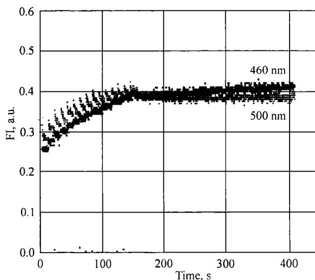
Fig. 1. The change of dansylamide fluorescence intensity (FI) recorded during the polymerization of TMPTMA/VP (9:1) mixture using photoinitiation system: RBAX ( $10 \cdot 10^{-4}$  M), NPG (0.05 M); mode of irradiation: LRS (0.2 s—10 s—0.2 s—10 s...), 15 flashes, total time irradiation 3 s, 600 mW/1.54 mm<sup>2</sup>,  $\lambda = 514$  nm
