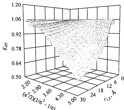
Fig. 6. Electron transfer process equilibrium constant  $K_{ET}$  versus the properties of solvent  $[(e^2/2)(1/n^2 - 1/\epsilon)]$  and distance separating the donor and acceptor molecules ( $r_{12}$ )
