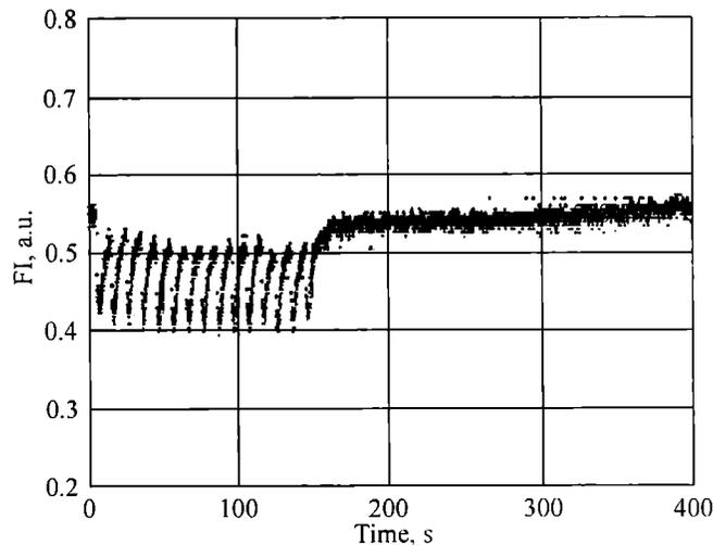
Fig. 5. The change of densylamide fluorescence intensity (FI) recorded during and after laser irradiation of TMPTMA/VP (9:1) mixture; initiation system: PG-Poly-OC(O)-RB-OAc ( $5 \cdot 10^{-4}$  M of RB); mode of irradiation — see Fig. 1
