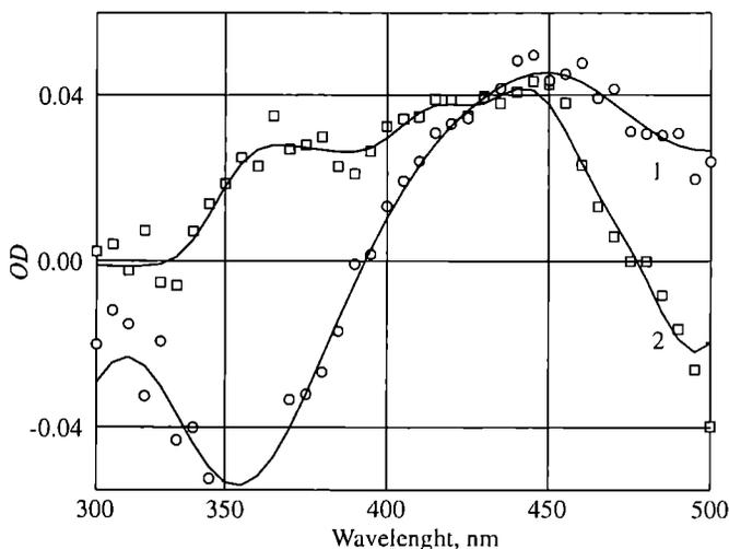
Fig. 9. Transient absorption spectra recorded  $6 \mu\text{s}$  after the laser flash for selected A-S-D photoinitiating systems in MeCN; 1 — PDRB, 2 — HDRB
