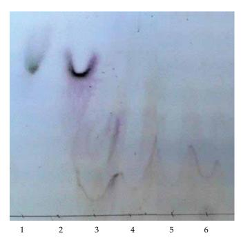
Fig. 6. A chromatogram of a 20-fold concentrated SBF fluid after BNC incubation in the presence of A. fumigatus for: 3-1 month, 4-2 months, 5-5 months, 6-6 months; 1- glucose reference, 2- cellobiose reference
