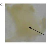
Fig. 2. Pictures of BNC samples: A) not incubated, B) incubated for 2 months, C) incubated for 3 months; arrows show brighter regions in the membrane that indicate a reduction of its thickness due to degradation
