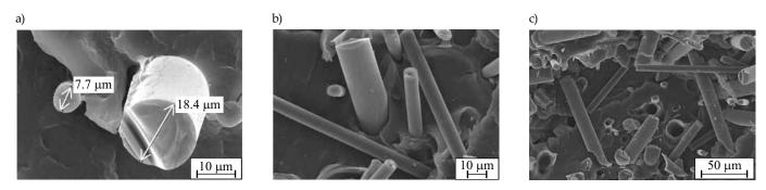
Fig. 2. SEM micrographs of tensile fractured surfaces of composites: a) PP5B5C, b) PP7B7C, c) PP10B10C
