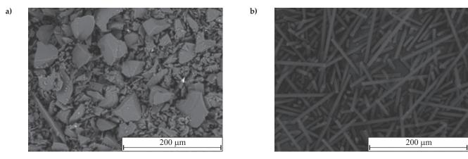
Fig. 7. SEM pictures of the particles of: a) glass frit, b) carbon fibers
