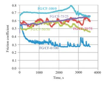
Fig. 5. Change in friction coefficient of the PUUR and composites during the test
