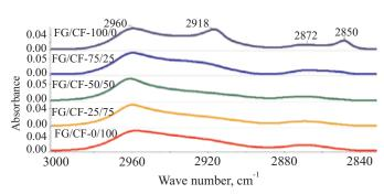
Fig 4. Part of FT-IR composite spectra within the range of 2840–3000 cm<sup>-1</sup> of the PUUR and composites
