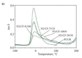
Fig. 3. Results of ureaurethane and composites analysis with DMA: a) storage modulus E', b) tan  $\delta$
