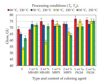
Fig. 5. Gloss values of ABS injection molded parts in a function of coloring agents, gloss examined at the light incidence on the molding surface in the direction opposite to the polymer flow in the cavity, 60° angle of the light incidence
