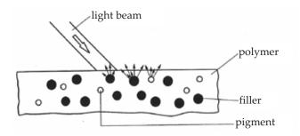
Fig. 1. Diagram of internally diffused light deflection (according [1])
