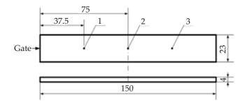
Fig. 2. Injection molded part with color measurement points
