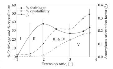
Fig. 2. Dependence of the degree of crystallinity, the measure of the amorphous phase orientation and the degree of shrinkage on the degree of deformation of the PET sample during uniaxial stretching at 2/s, at a constant temperature of 100°C, divided into five individual stages of shrinkage response [41]
