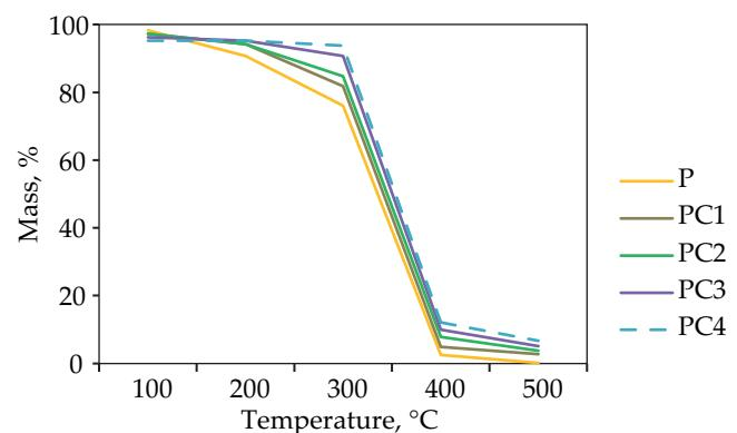
Fig. 6. TGA curves of PLA biocomposites
