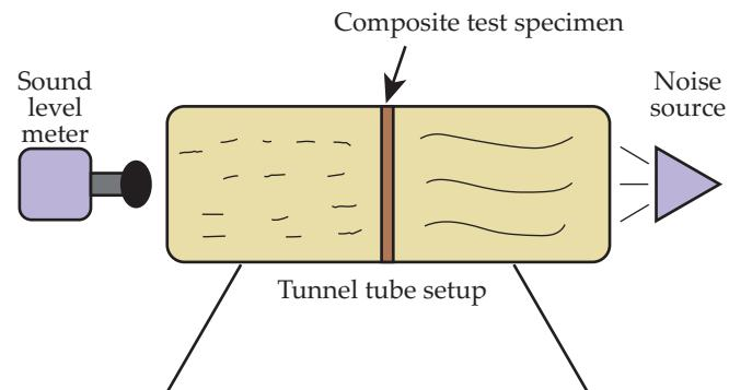
**Fig. 1. Sound test impedance tube**
