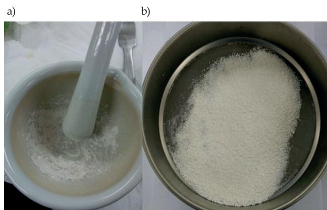
Fig. 4. Grinding of dried Nata de Coco powder (a), sieving of BC mech powder (b)
