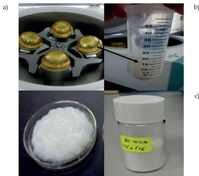
Fig. 3. Centrifuge machine (a), supernatant precipitate (b), dried powder of chemically treated BC (c)
