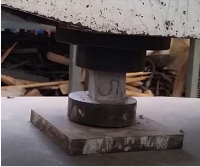
Fig. 8. Mortar cubes for compression testing
