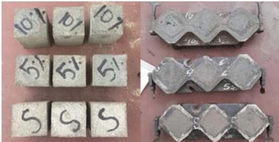
Fig. 6. Cube samples for compressive strength test of mortar
