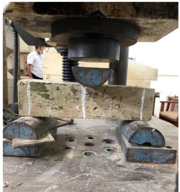
Fig. 10. Concrete prism for flexural testing
