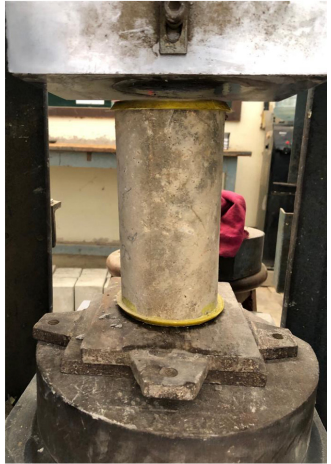
Fig. 9. Concrete cylinder for compression testing
