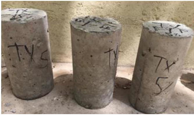
Fig. 4. Cylinder samples for compressive strength test of concrete
