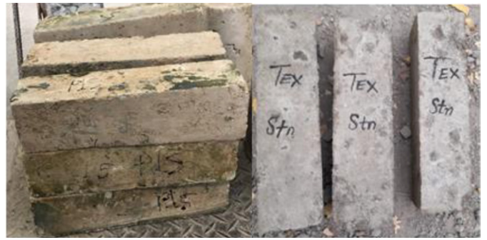
Fig. 5. Prisms samples for flexural strength test of concrete
