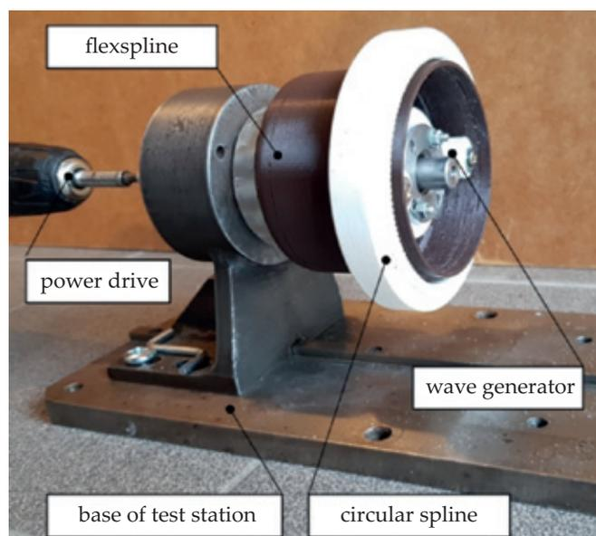
Fig. 1. Station designed for testing the harmonic drives
