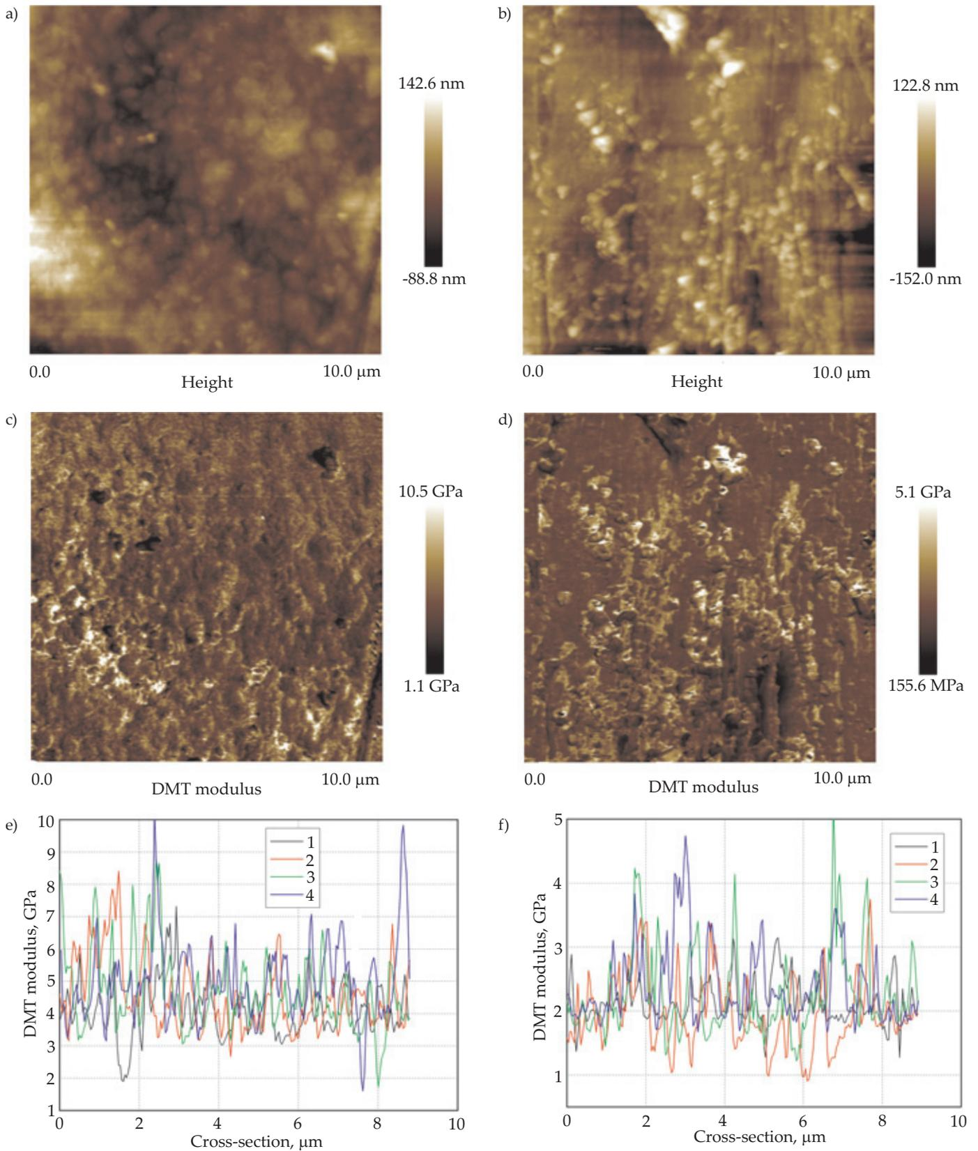
**Fig. 5.** AFM images showing topography and distribution of Young DMT modulus in the surface of gear wheel teeth made of PLA: a, c, e) before the cycle of operation and accelerated aging, b, d, f) following 150 cycles of operation and the aging procedure
