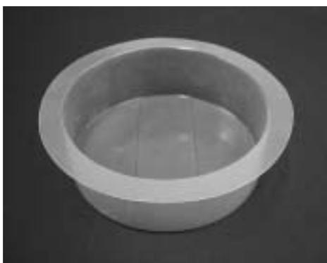
Fig. 1. General view of the thermoformed container with circular cross-section
