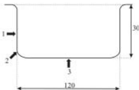
Fig. 2. Approximate sites of the measurements of the wall thickness of the containers studied: 1 — side wall, 2 — area of transition between the side wall and the bottom, 3 — bottom
