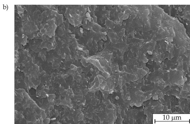
Fig. 6. SEM analysis of PA6 filled with hybrid flame retardant synthesized: a) in the presence of PVA, b) in the absence of PVA
