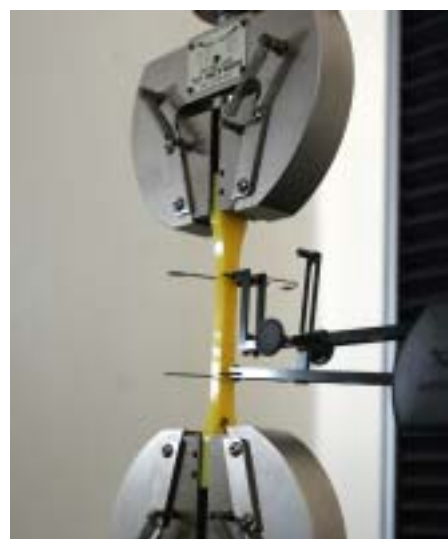
Fig. 1. View of sample during test using tensile testing machine with the use of DA extensometer
