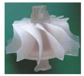
*Fig. 3. Appearance of an impeller obtained from composite based on Polimal*® 109-32 *RPyK with* 1.5 *phr of BS modified with QAS2*
