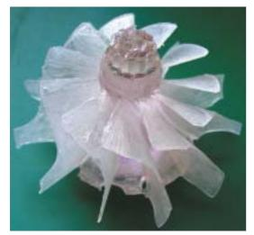
Fig. 2. Appearance of an impeller obtained from composite based on Polimal® 109-32 RPyK with 3 phr of BS modified with QAS2
