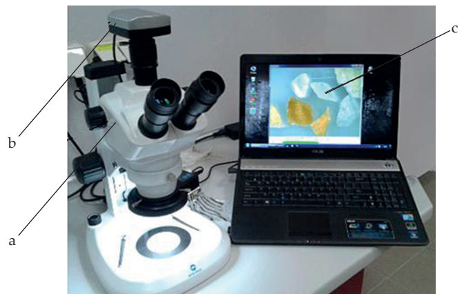
Fig. 2. Image recording and analysis: a) stereo microscope, b) digital camera, c) computer software
