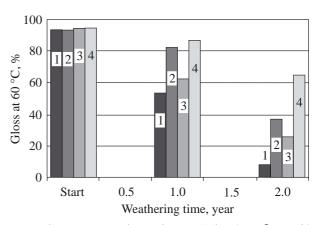
Fig. 3. Gloss at natural weathering (Florida  $45^{\circ}$  South) of epoxy acrylic silicone hybrid coatings based on epoxy functional polysiloxane and acidic functional acrylic resin (3 not washed, 4 — washed) in comparison with polyurethane (1 — not washed, 2 — washed)
