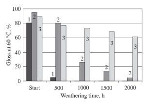
*Fig. 1. Artificial QUV-B weathering of epoxyamine silicone hybrid coating (3) in comparison with control samples: epoxy amine (1) and polyurethane (2)*
