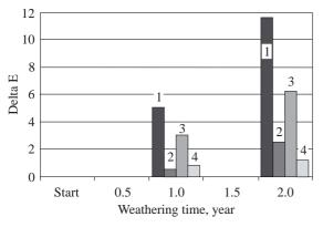
Fig. 4. Colour change (delta E) at natural weathering (Florida 45° South) of epoxy acrylic silicone hybrid coatings based on epoxy functional polysiloxane and acidic functional acrylic resin (3 — not washed, 4 — washed) in comparison with polyurethane (1 — not washed, 2 — washed)
