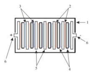
Fig. 1. Cross-section of a bipolar lead-acid battery: 1 - container, 2 - positive active mass (PAM) on one face, <math>3 - negative active mass (NAM) on the other face, 4 - glass fibre separator, 5 - support, 6 - monopoles
