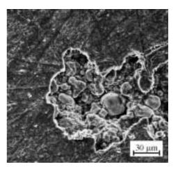
Fig. 4. Surface of the composite with 94 wt. % content of BMP
