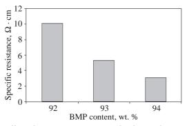
*Fig. 3. Effect of BMP content on specific electrical resistance of the blend*
