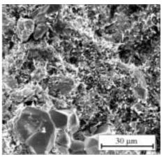
Fig. 5. Cross-section of the composite with 94 wt. % content of BMP
