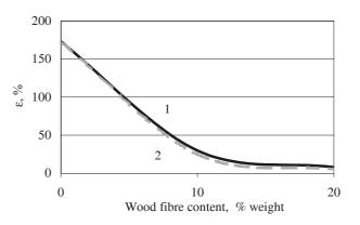
*Fig.* 3. Comparison of elongation at break ( $\varepsilon$ ) of the composites of recycled PP with different content and type of wood flour, 1 — PP with CB 120, 2 — PP with BK 40/90
