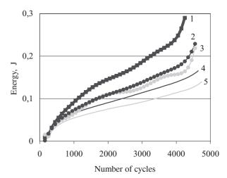
*Fig. 8. Influence of wood flour on dissipation of mechanical energy of PP composites; for symbols — see Fig. 5*
