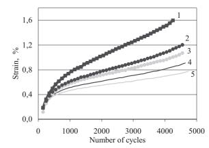
*Fig. 7. Comparison of strain under cyclic loading of PP composites with two types of wood flour; for symbols — see Fig. 5*
