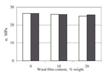
Fig. 2. Comparison of tensile strength ( $\sigma_M$ ) of the composites of recycled PP with different content and type of wood flour;  $\Box - CB \ 120, \blacksquare - BK \ 40/90$
