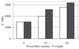
Fig. 1. Comparison of tensile modulus (E) of the composites of recycled PP with different content and type of wood flour;  $\Box$  — CB 120,  $\blacksquare$  — BK 40/90
