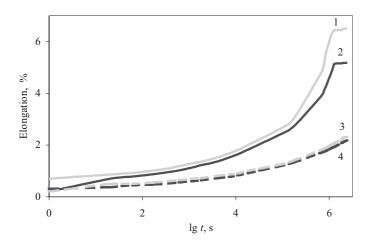
Fig. 4. Creep curves, illustrating the dependence of elongation on time (t), for recycled PP filled with wood flour: 1 - PP + 10% of CB 120, 2 - PP + 10% of BK 40/90, 3 - PP + 20%of CB 120, 4 - PP + 20% of BK 40/90
