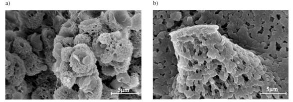
Fig. 9. SEM images: a) PP, b) single particle in polymer matrix; magnification 5000 times
