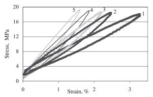
*Fig. 5. Examples of hysteresis loops of PP composites with two different types of wood flour (first cycle):* 1 — *PP,* 2 — *PP with 10 % of BK 40/90,* 3 — *PP with 10 % of CB 120,* 4 — *PP with 20 % of BK 40/90,* 5 — *PP with 20 % of CB 120*
