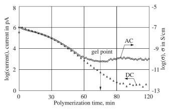
Fig. 4. Comparison of the evolution of logarithm of the isochronal current values after 10 s of charging (DC measurements, Ni electrodes IDEX sensor, polarization time 90 s, U = 5 V) and of the AC conductivity (dielectric measurements, Ni electrodes IDEX sensor, 20 Hz, U = 5 V) for the DGEBA-3DCM system isothermally cured at 70 °C
