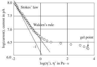
Fig. 8. Relationship between the logarithmic values of the ionic current (DC measurements, Cu sandwich-type electrodes, d = 0.080 mm, 10 s, U = 1 V) and of the dynamic viscosity  $\eta'$  (DMA measurements, plates 40 mm, 0.16—16 Hz) for the DGEBD-4D system isothermally cured at 50 °C; the lower line indicates a slope of -1
