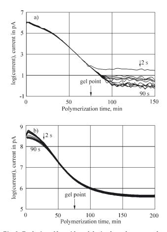
Fig. 3. Evolution of logarithm of the isochronal current values measured after different times of polarisation (2—90 s of charging) during isothermal cure of: a) the DGEBA-3DCM system at 70 °C (DC measurements, Ni electrodes IDEX sensor, polarization time 90 s, U = 5 V), b) DGEBD-4D system at 60 °C (DC measurements, parallel sandwich-type Cu electrodes, d = 0.080 mm, polarization time 90 s, U = 1 V)
