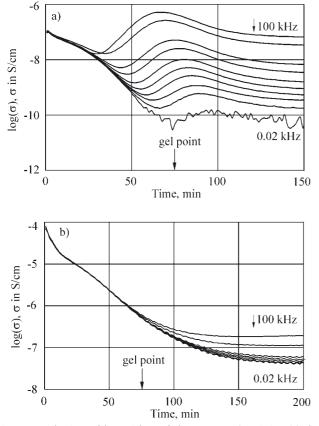
Fig. 2. Evolution of logarithm of the AC conductivity (dielectric measurements, Ni electrodes IDEX sensor, frequency was equal 0.02, 0.1, 0.2, 0.5, 2, 5, 10, 50 or 100 Hz, U = 5 V), obtained for: a) DGEBA-3DCM system isothermally cured at 70 °C, b) DGEBD-4D system isothermally cured at 60 °C
