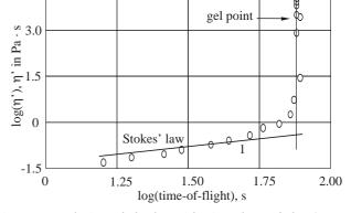
Fig. 7. Correlation of the logarithmic values of the dynamic viscosity  $\eta'$  (DMA measurements, plates 40 mm, 0.16— 16 Hz) and of the time-of-flight of ions  $\tau_i$  (TOF experiment, Au electrodes IDEX sensor, U = 5 V) for the isothermal cure of the DGEBD-4D system at 50 °C; line with a slope of 1 indicates the Stokes law
