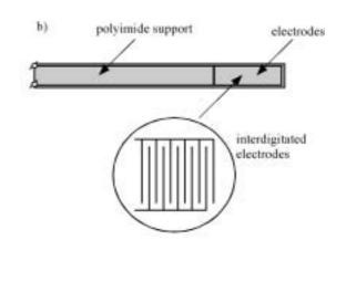
*Fig.* 1. *Schemes of: a) the AC, DC and TOF measurement circuits, b) the IDEX sensor, c) the sandwich-type configura-tion of the electrodes*
