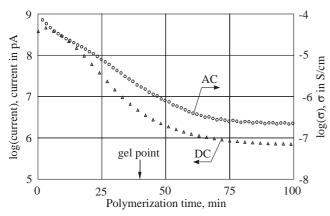
Fig. 5. Comparison of the evolution of logarithm of the isochronal current values after 10 s of charging (DC measurements, parallel sandwich-type Cu electrodes, d = 0.080 mm, polarization time 90 s, U = 1 V) and of the AC conductivity (AC measurements, Ni electrodes IDEX sensor, 20 Hz, U = 1 V) for the DGEBD-4D system isothermally cured at 70 °C
