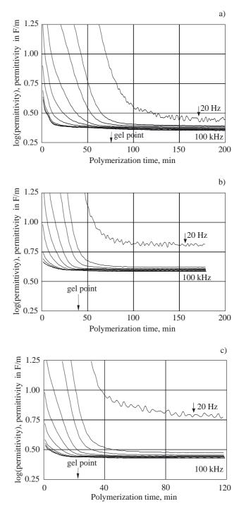
Fig. 9. Evolution of logarithm of permittivity (AC measurements, Ni electrodes Idex sensor, 20Hz—100kHz, U = 1V) during the cure of the DGEBD-4D system at a) 60 °C, b) 70 °C, c) 80 °C
