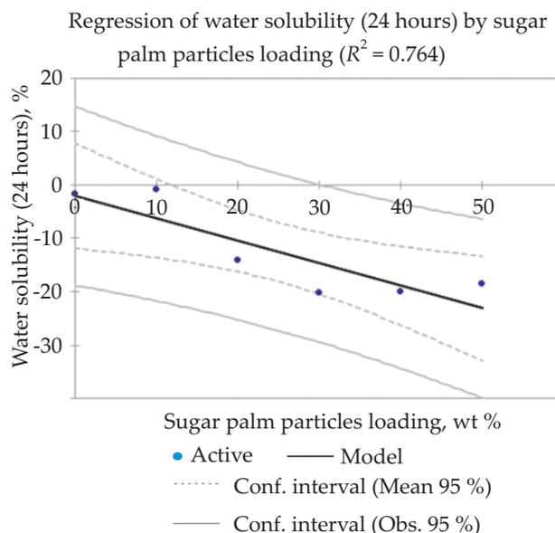
**Fig. 5.** Water solubility for 24 hours as a function of sugar palm particles loading (0–50 wt %)**Table 9.** Correlation between water solubility and sugar palm particles loading (0–50 wt %)
