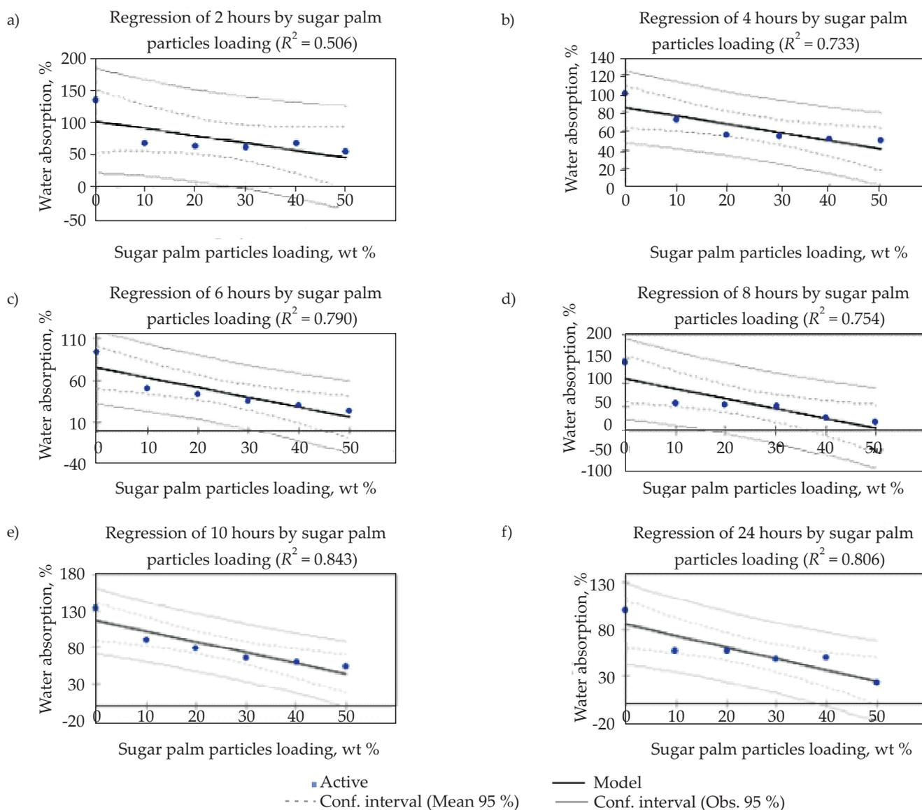
Fig. 4. Water absorption after 2, 4, 6, 8, 10 and 24 hours of immersion as a function of sugar palm particles loading (0–50 wt %)
