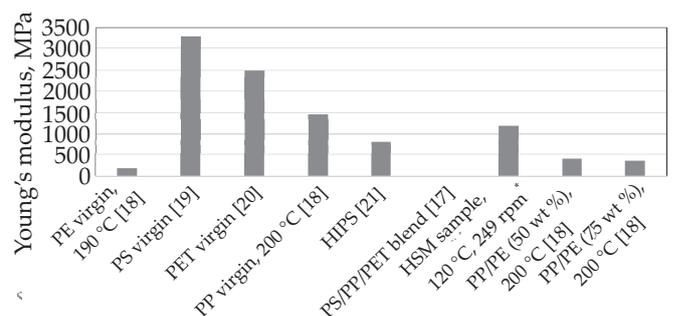
Fig. 4. Comparison of Young's modulus for different type of polymers
