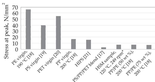
Fig. 2. Comparison of stress at peak for different type of polymers
