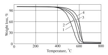
*Fig. 1. TGA curves of PP compositions: 1 — MH1, 2 — MH2, 3 — MH3, 4 — MH4*
