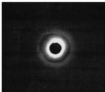
Fig. 4. WAXS pattern of 2,7-DGEDHN/DAF mixture
