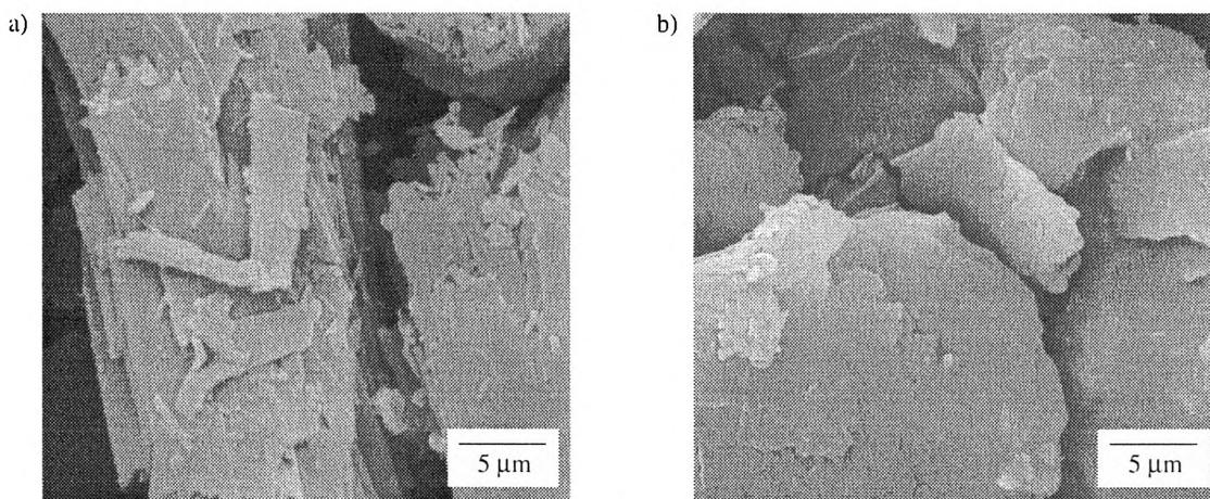
Fig. 6. SEM micrographs of LiCMC (a) and NaCMC (b) modified products with HDI
