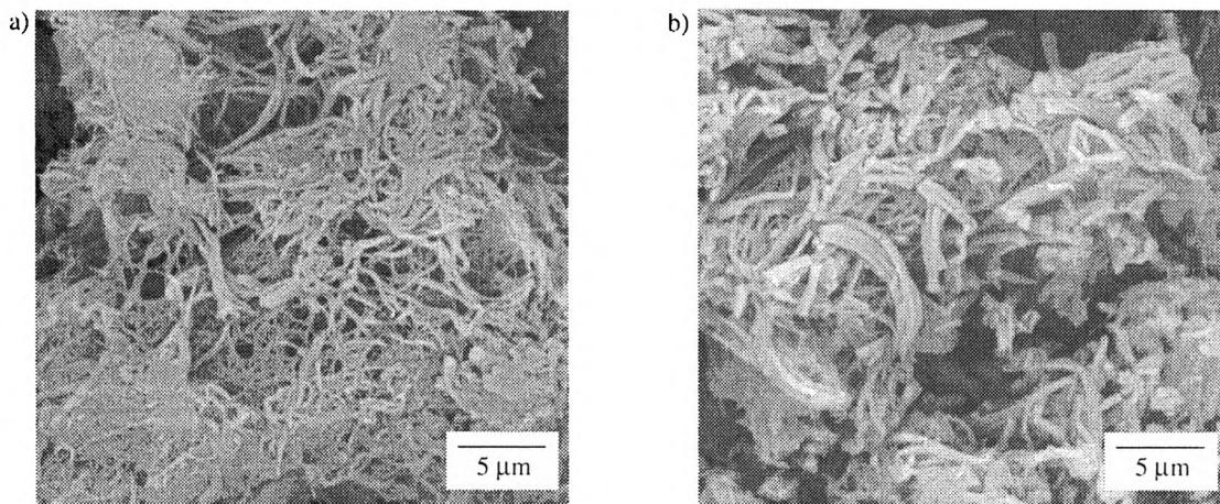
Fig. 5. SEM micrographs of LiCMC (a) and NaCMC (b) modified products with OctI
