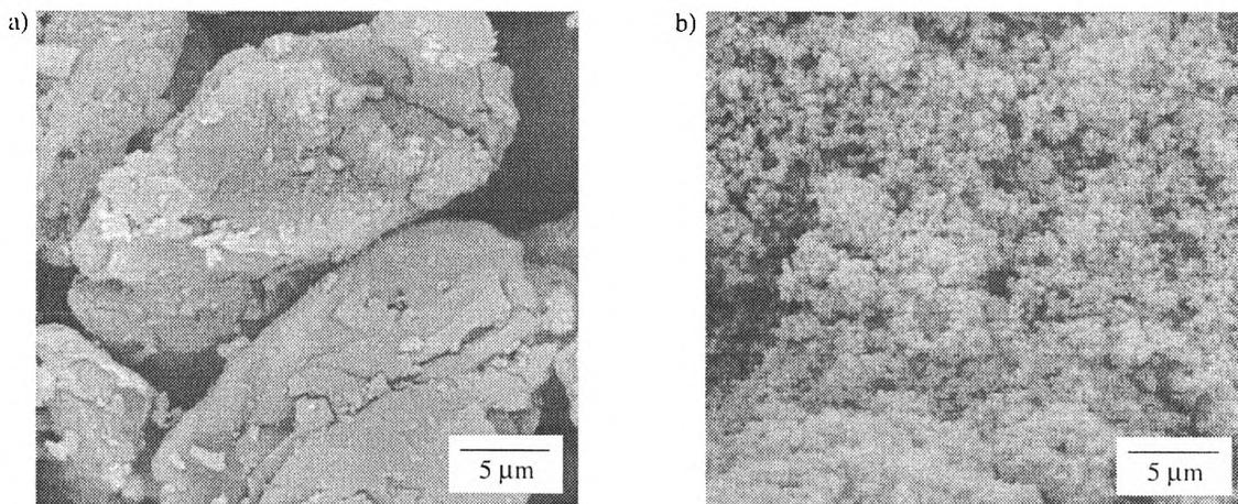
Fig. 4. SEM micrographs of LiCMC (a) and NaCMC (b)
