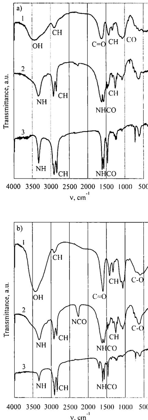
Fig. 1. Infrared spectroscopy of LiCMC (a) and NaCMC (b) and their modified products; LiCMC or NaCMC: pure — curves 1, with HDI — curves 2, with OctI — curves 3
