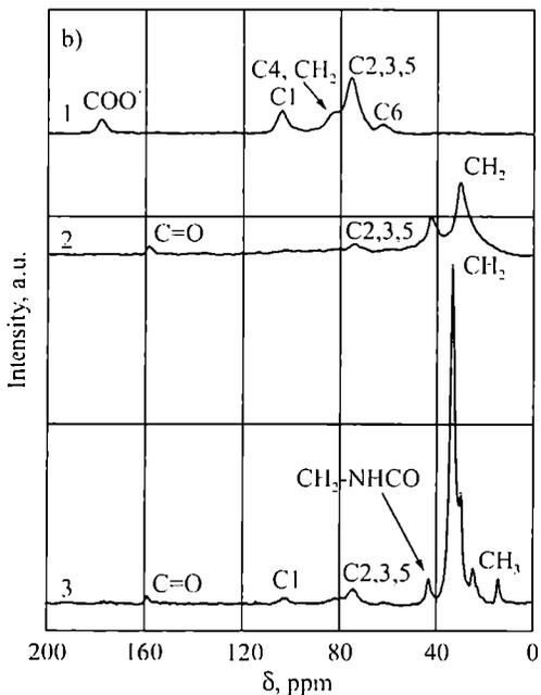
Fig. 2. Solid state  $^{13}\text{C}$  NMR spectra of LiCMC (a) and NaCMC (b) and their modified products; LiCMC or NaCMC: pure — curves 1, with HDI — curves 2, with OctI — curves 3
