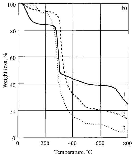
Fig. 3. TGA measurements of LiCMC (a) and NaCMC (b) and their modified products; LiCMC or NaCMC: pure — curves 1, with HDI — curves 2, with OctI — curves 3
