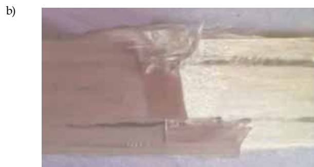
Fig. 10. Images of a sample after impact resistance determination: a) PET-G, b) specimen E (composite PET-G with 20 wt % of PET)
