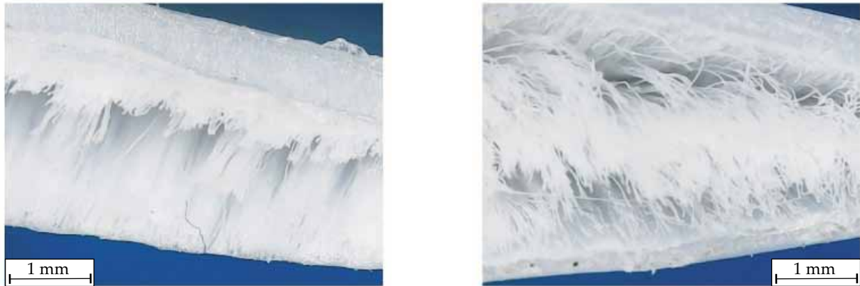
Fig. 8. Examples of delamination of composite materials (with 15 wt % content of reinforcement) resulting from the action of boiling water
