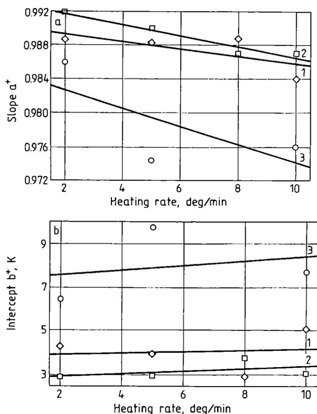
Fig. 5. Slope  $a^+$  (a) and intercept  $b^+$  (b) of the plot of true melting temperature  $T_i^+$  vs. measured values  $T_m$  using indium and tin samples of various masses (mg): 1 — 3.5, 2 — 7.5, 3 — 10
