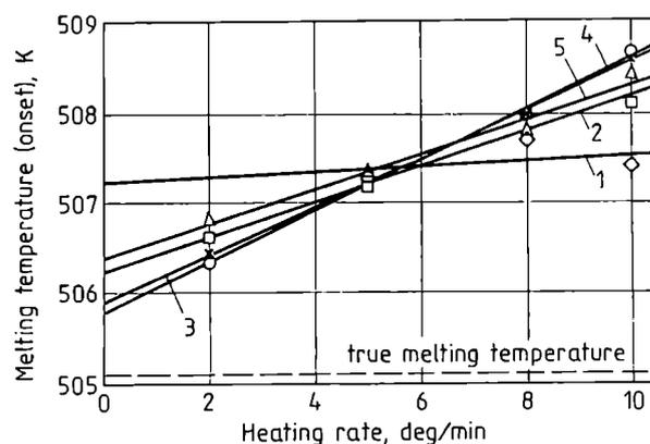
Fig. 2. Measured melting temperature of tin vs. heating rate at various sample masses (mg): 1 — 0.98, 2 — 3.30, 3 — 5.79, 4 — 7.49, 5 — 9.86
