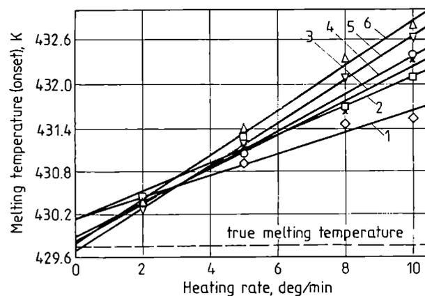
Fig. 1. Measured melting temperature of indium vs. heating rate at various sample masses (mg): 1 — 3.42, 2 — 5.11, 3 — 7.57, 4 — 10.63, 5 — 14.29, 6 — 19.40
