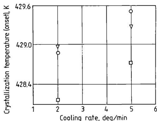
Fig. 7. Effect of sample mass on the corrected temperature of indium crystallization on cooling without nitrogen; sample mass (mg):  $\square$  — 3.2,  $\circ$  — 7.57,  $\nabla$  — 10.63
