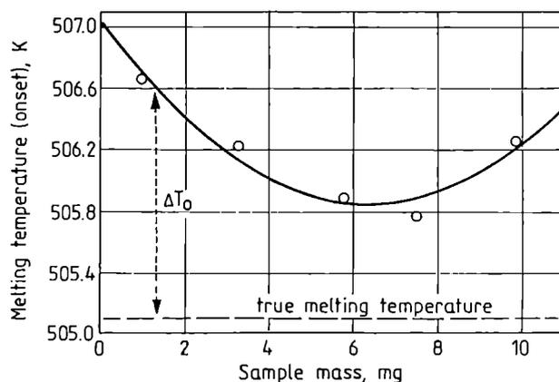
Fig. 4. Melting temperature of tin extrapolated to zero heating rate vs. sample mass
