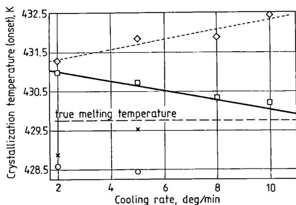
Fig. 6. Measured and corrected temperatures (onset) of indium (7.57 mg) on cooling with and without liquid nitrogen;  $\square$  and  $\diamond$  — temperatures measured and corrected, resp.; liquid nitrogen used as coolant  $\circ$  and  $\times$  — temperatures measured and corrected, resp.; no liquid nitrogen used as coolant
