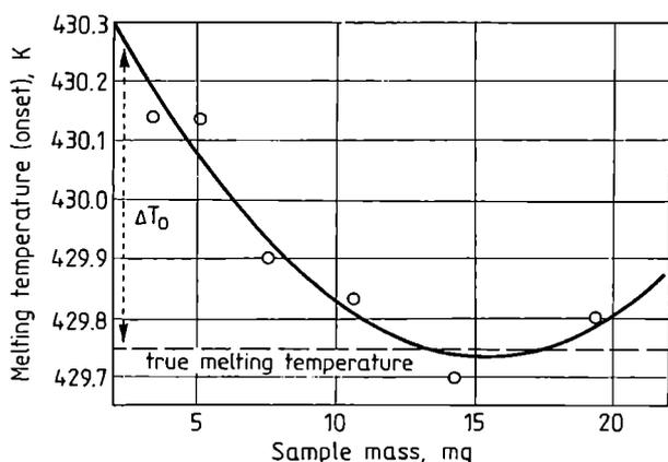
Fig. 3. Melting temperature of indium extrapolated to zero heating rate vs. sample mass
