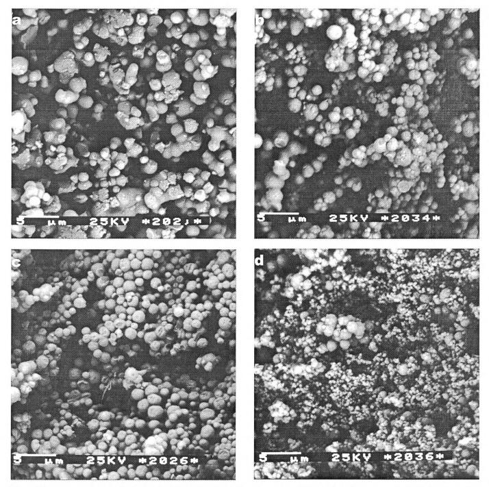
Fig. 3. SEM photomicrographs (4000×) of poly(AMA/MMA) microspheres obtained by dispersion polymerization in methanol in the presence of 5% of MPEGMA: (a) MPEGMA 550, (b) MPEGMA 750, (c) MPEGMA 2000, (d) MPEGMA 5000
