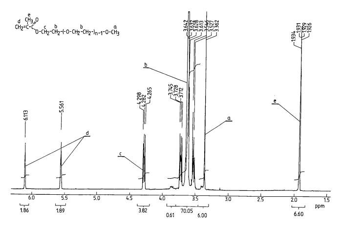
Fig. 2. <sup>1</sup>H-NMR spectrum of MPEGMA 550
