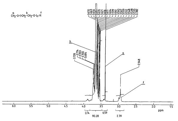
Fig. 1. <sup>1</sup>H-NMR spectrum of MPEG 550
