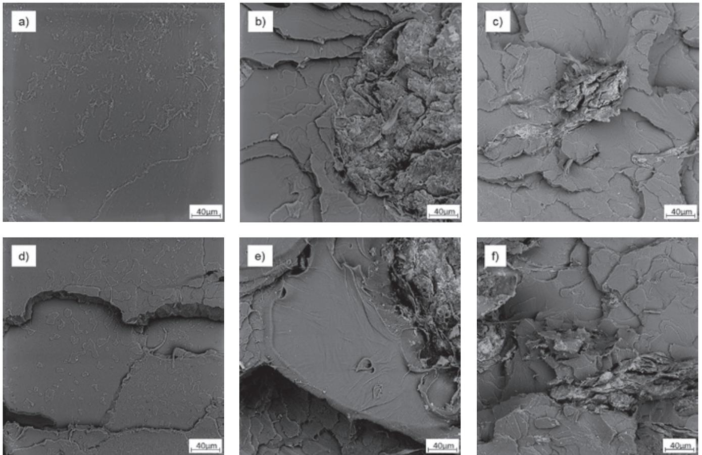
Fig. 7. SEM images of PLA/NC composites after impact test: a) 0 wt%NC, b) 3 wt% NC, c) 5 wt% NC, and after tensile test: d) 0 wt% NC, e) 3 wt% NC, f) 5 wt% NC
