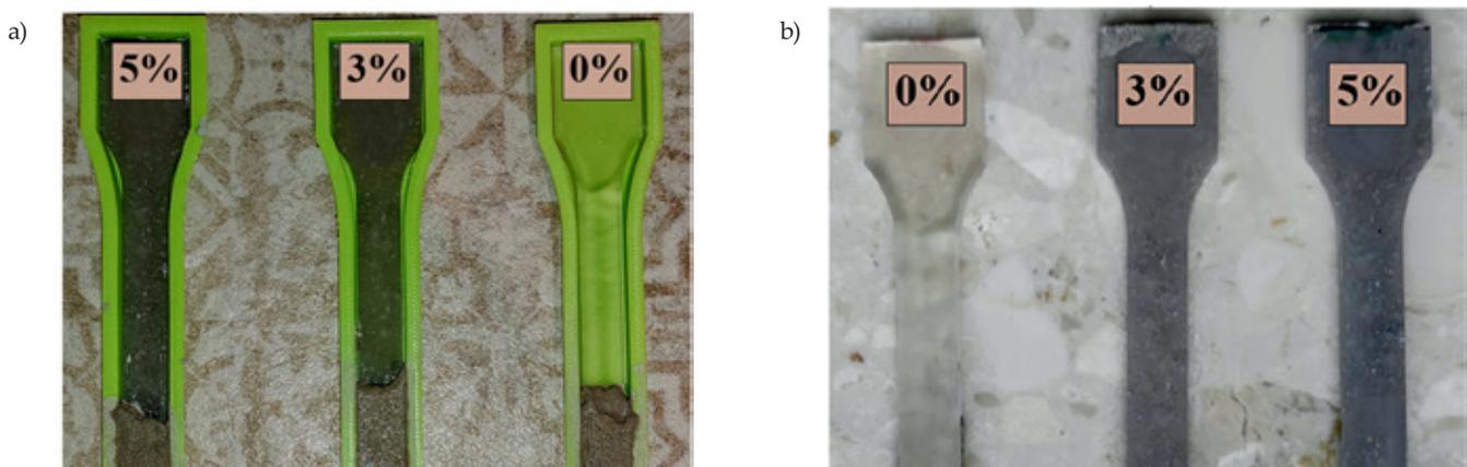
Fig. 8. Appearance of the samples before (a) and after (b) the adhesion test
