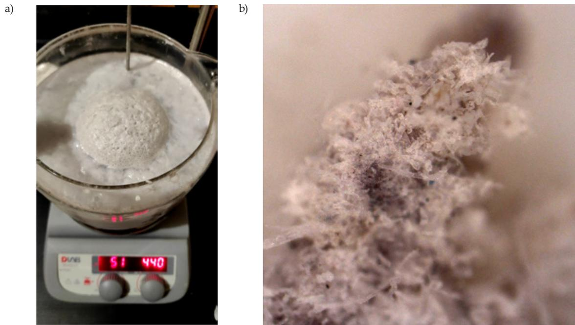
Fig. 2. Cellulose pulp (a), fibrillar nanocellulose (b)
