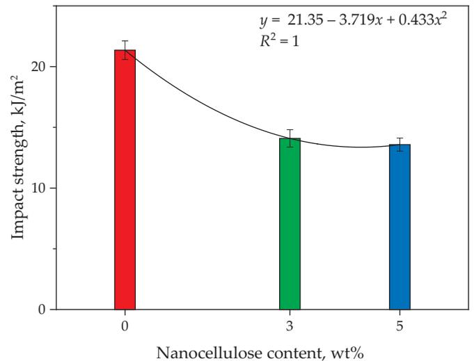
Fig. 5. Impact strength of PLA/NC composites
