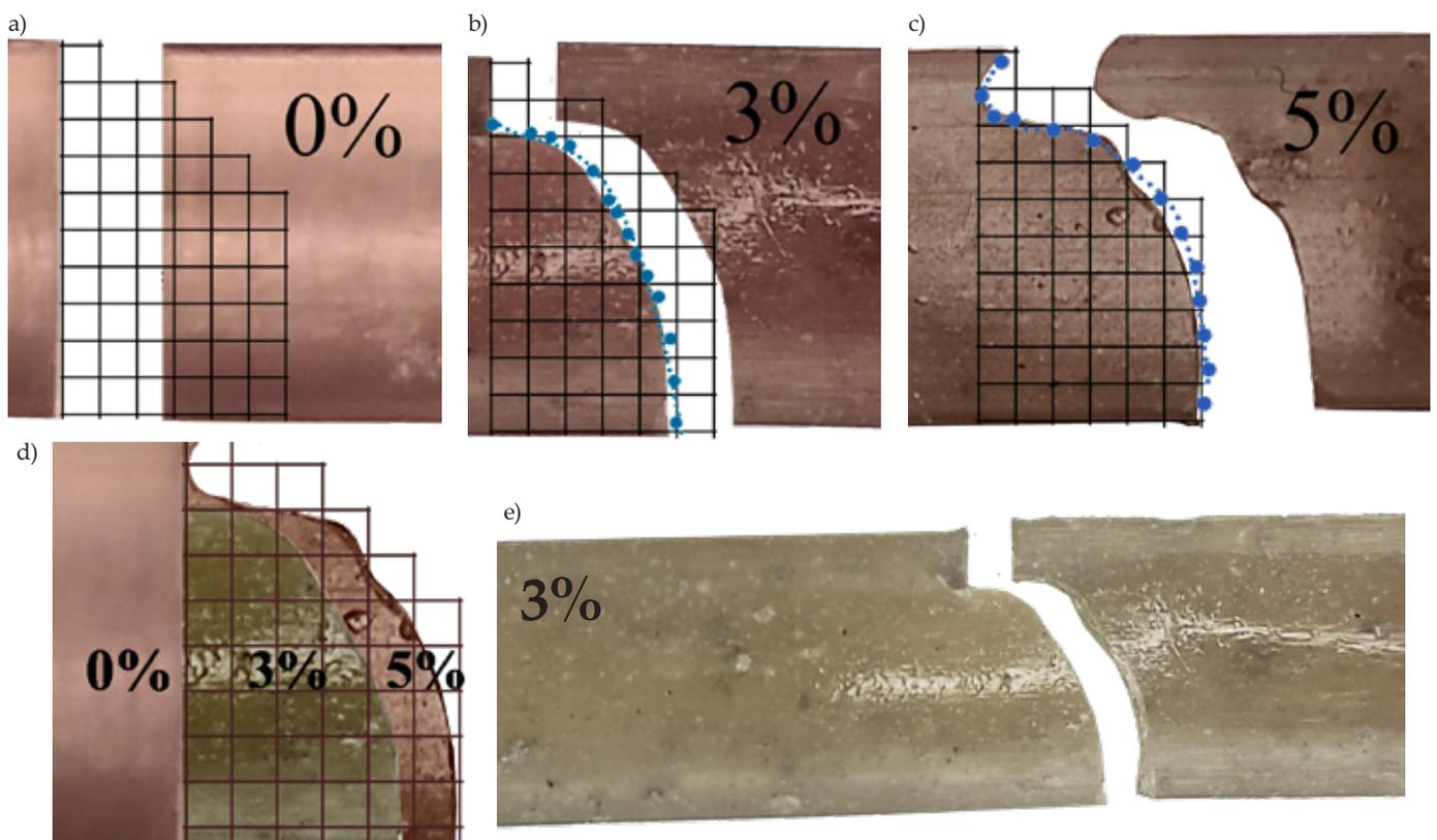
Fig. 3. The method of evaluating PLA/NC impact resistance: a) 0 wt% NC, b) 3 wt% NC, c) 5 wt% NC, d) comparison of all samples, e) 3 wt% NC (the whole sample after the test)
