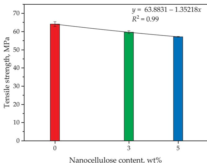
Fig. 6. Tensile strength of PLA/NC composites
