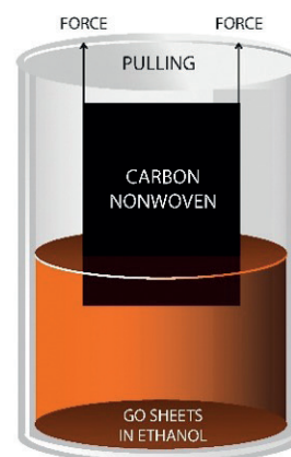
Fig. 6. Scheme of the dip-coating process
