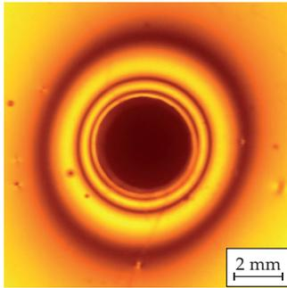
Fig. 1. Interference fringes for Ortho Connect material
