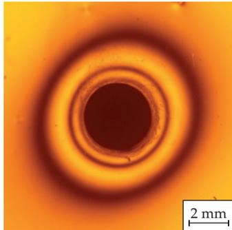
Fig. 3. Interference fringes for Transbond XT material
