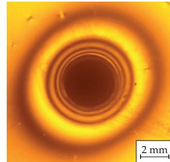
Fig. 4. Interference fringes for Resilience material
