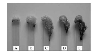
Fig. 3. Photographs of PMMA-based samples after flammability tests: A – PMMA-0, B – PMMA-1, C – PMMA-5, D – PMMA-7.5, E – PMMA-10 [10]
