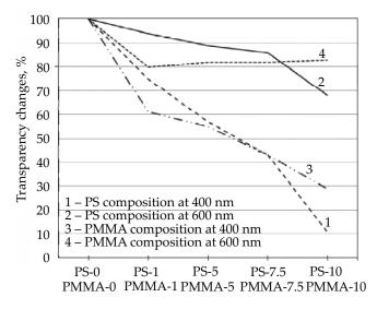
Fig. 4. Influence of DOPO addition on transparency of polystyrene (PS) and poly(methyl methacrylate) (PMMA)
