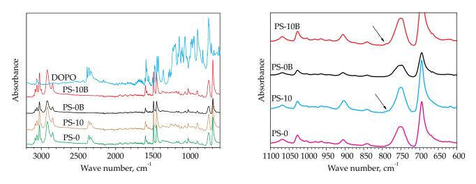
Fig. 1. FT-IR spectra for DOPO, PS-0, PS-10 compositions and burn residues of these materials (PS-0B and PS-10B)
