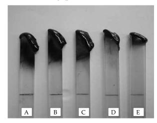
Fig. 2. Photographs of PS-based samples after flammability tests: A – PS-0, B – PS-1, C – PS-5, D – PS-7.5, E – PS-10
