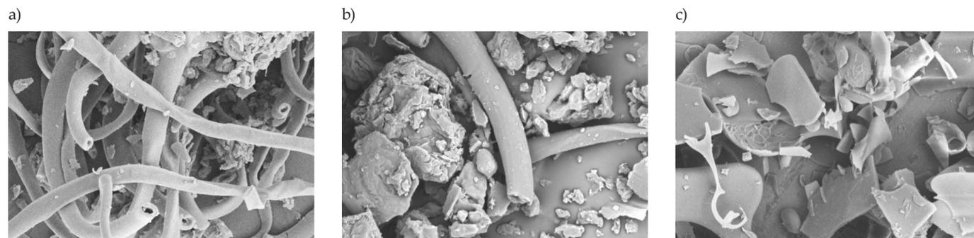
Fig. 3. Images of sage fillers at a magnification of 2500 $\times$ : a) before modification, b) after modification, c) polyphenolic extract
