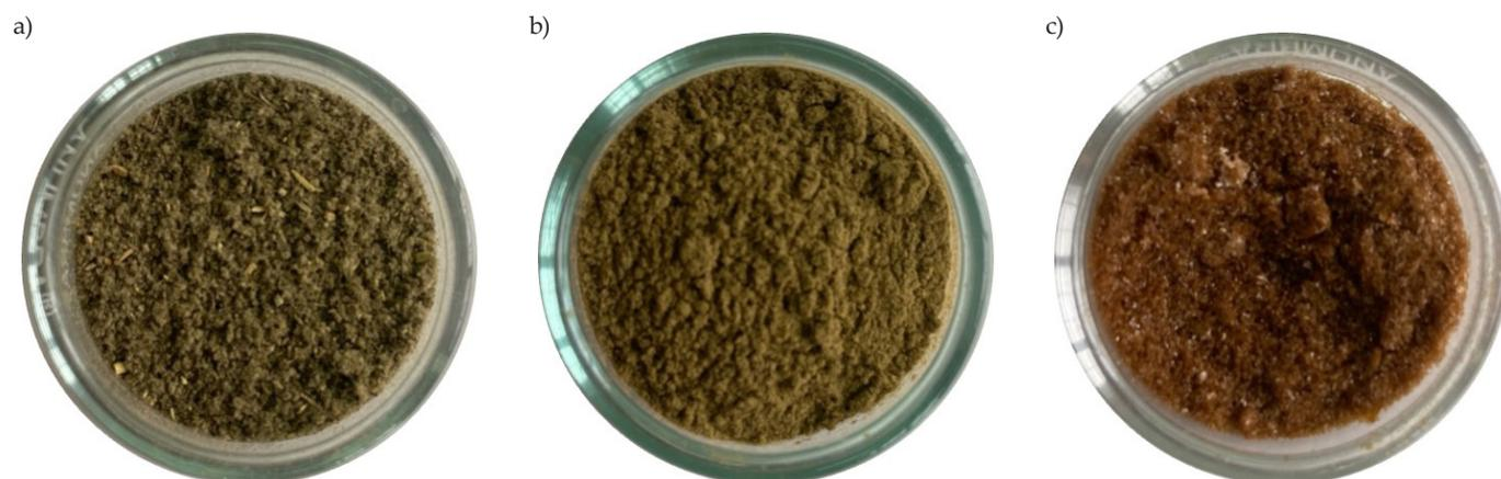
Fig. 1. Tested fillers: a) raw sage, b) modified sage, c) sage extract
