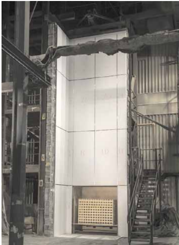
Fig. 3. The test rig for the fire test BS8414 (from https://www.gov.uk/government/uploads/system/uploads/attachment_data/file/639357/DCLGtest7_BS8414_Part_1_test_report_Issue_2_0.pdf )
