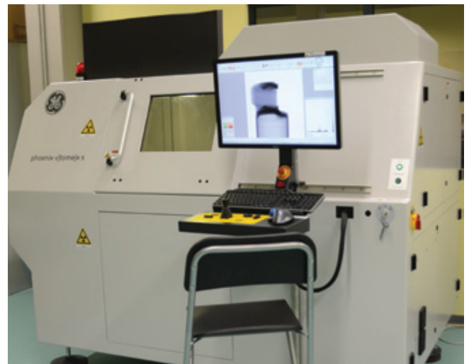
Fig. 3. Micro CT equipment type GE Phoenix v|tome|x s240 used for research
