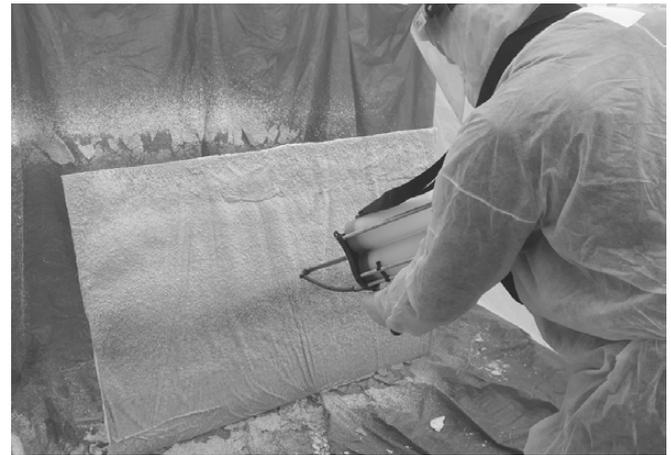
Fig. 2. Preparation of polyurea spray coatings
