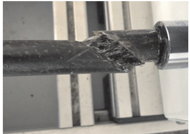
Fig. 7. The failure test result of the non-hybrid epoxy composites reinforced with 20 wt % of sugar palm fiber
