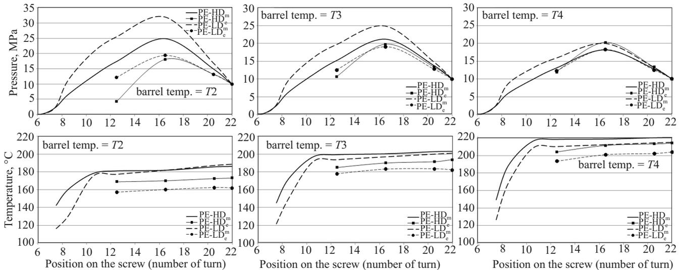
Fig. 9. The pressure profiles (top) and temperature profiles (bottom) of the plastication process for PE-LD and PE-HD at different barrel temperatures
