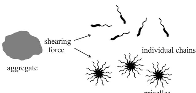
Fig. 2. Behavior of poly(2-ethyl-2-oxazoline)-block-poly(2-phenyl-2-oxazoline) aggregates in water under the action of shear forces
