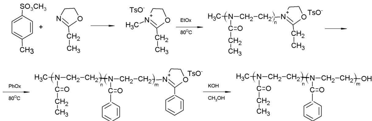
Scheme C. Synthesis of poly(2-ethyl-2-oxazoline)-block-poly(2-phenyl-2-oxazoline) ( $n = 60$ ,  $m = 4, 12, 37$ )
