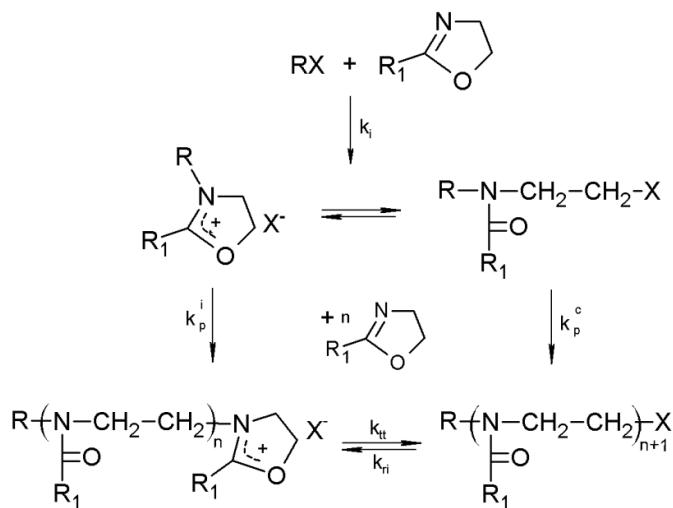
Scheme A. Polymerization of 2-oxazolines
