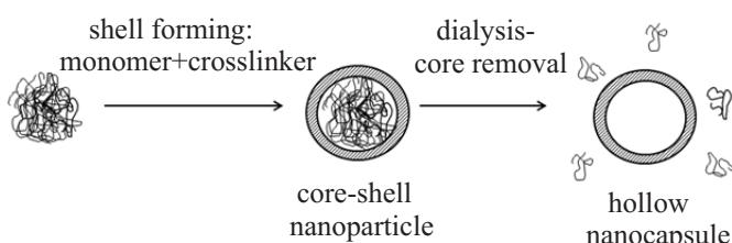
Fig. 6. The route to hollow nanoparticles using thermoresponsive template
