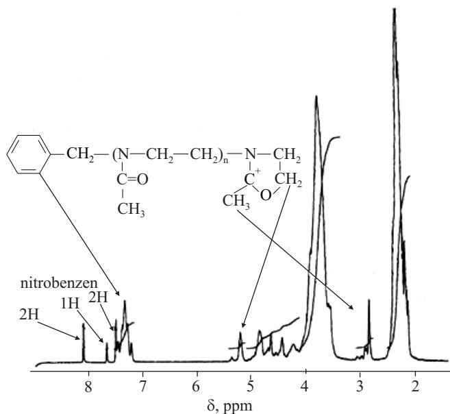
Fig. 1.  $^1\text{H}$  NMR (600 MHz) spectrum of the living polymer of methyl oxazoline (initiator benzyl bromide(I), solvent nitrobenzene,  $[M]_0 = 1.5 \text{ mol}/\text{dm}^3$ ,  $[I]_0 = 0.15 \text{ mol}/\text{dm}^3$ ,  $25^\circ\text{C}$ ) (according to [16])
