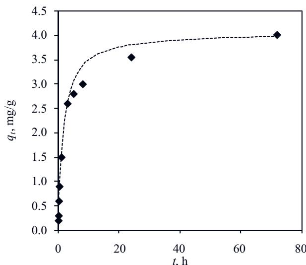
Fig. 1. Effect of time on Cr(VI) removal by hybrid polymer (1.0 g of R/S/Fe sample + 100 cm<sup>3</sup> K<sub>2</sub>CrO<sub>4</sub> solution [50 mg Cr(VI)/dm<sup>3</sup>]). Experimental data and pseudo-second order model calculations are represented by symbols and lines, respectively
