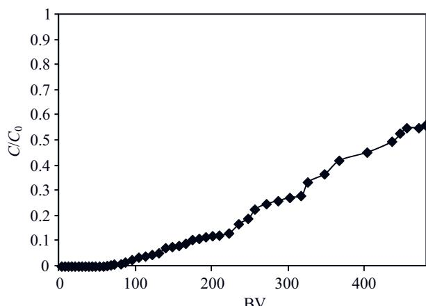
**Fig. 4.** Breakthrough curve for hybrid polymer R/S/Fe bed at  $10 \text{ mg Cr(VI)}/\text{dm}^3$  ( $\text{BV} = 15.5 \text{ cm}^3$ , flow rate  $3.5 \text{ BV/h}$ )
