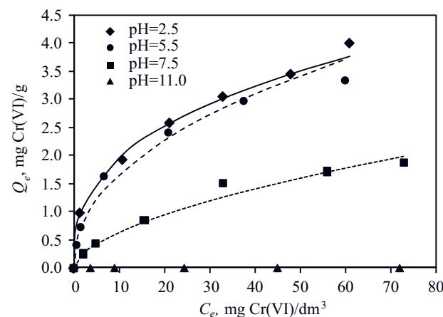
**Fig. 3.** The equilibrium chromate concentration ( $C_e$ ) versus the equilibrium adsorption capacity ( $Q_e$ ) for Cr(VI) adsorption by hybrid polymer R/S/Fe at varying pH of 2.5–11.0. Experimental data and Freundlich model calculations are represented by symbols and lines, respectively
