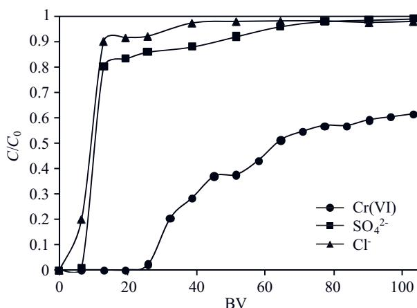
Fig. 6. Breakthrough curve for hybrid polymer bed at 10 mg Cr(VI)/dm<sup>3</sup>, 500 mg Cl<sup>-</sup>/dm<sup>3</sup> and 1000 mg SO<sub>4</sub><sup>2-</sup>/dm<sup>3</sup> (BV = 15.5 cm<sup>3</sup>, flow rate 3.5 BV/h)
