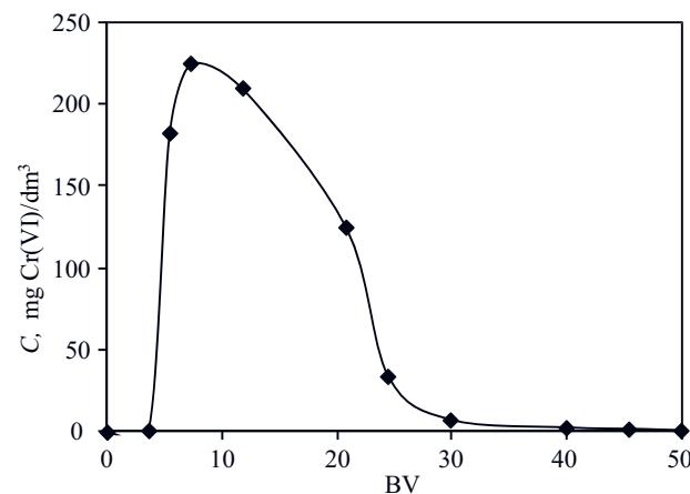
**Fig. 5.** Chromate elution curve ( $0.1 \text{ M NaOH}$  solution, flow rate  $3.5 \text{ BV/h}$ )
