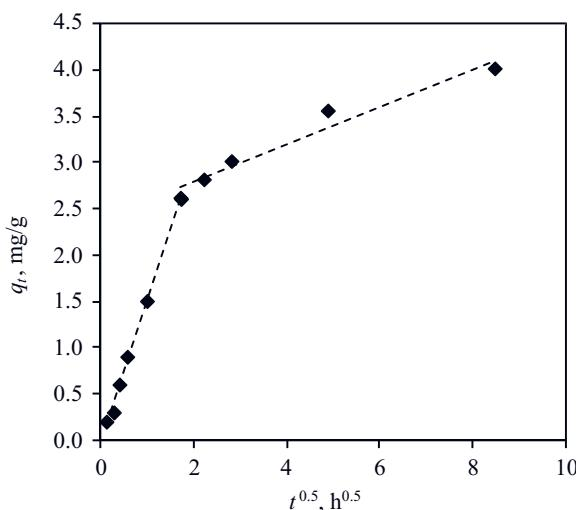
**Fig. 2.** Intraparticle diffusion plot for the removal of Cr(VI) by hybrid polymer [1.0 g of R/S/Fe sample + 100 cm<sup>3</sup> K<sub>2</sub>CrO<sub>4</sub> solution (50 mg Cr(VI)/dm<sup>3</sup>)]
