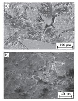
*Fig. 5. SEM images of the surface: a) bonded magnet, b) soft magnetic composite*
