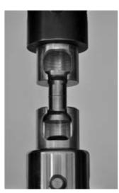
Fig. 3. A sample placed in the tensile test machine handles
