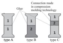
*Fig. 2. Three types of tested samples; designations of materials:* 1 - soft magnetic material, 2 - hard magnetic material
