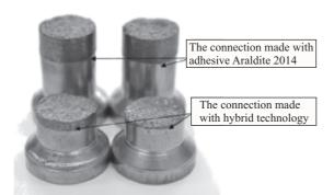
Fig. 8. Samples of type C after the strength tests
