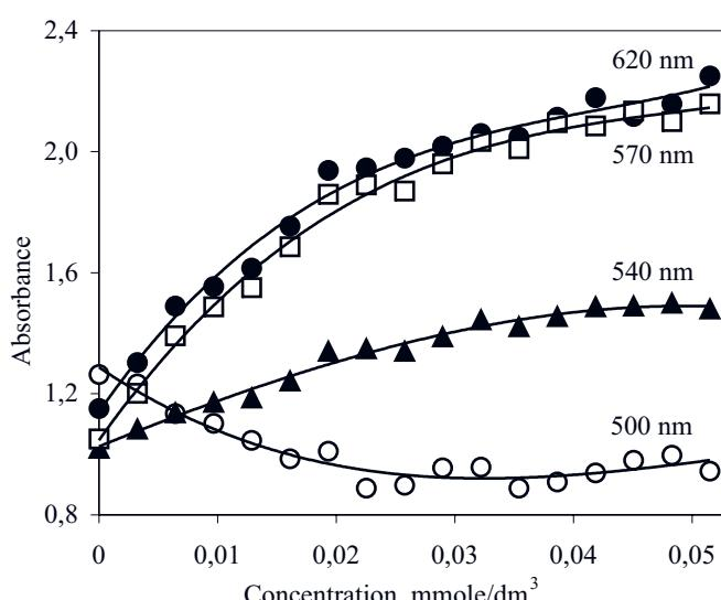
Fig. 2. Dependence of absorbance at different wavelengths on concentration of PDDA monomer units
