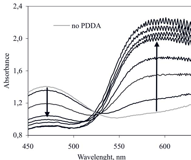
Fig. 1. Absorption spectra of CBB-PDDA complexes for increasing concentrations (in the direction of the arrows) of PDDA monomer units
