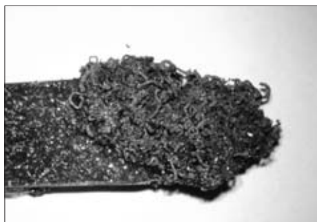
Fig. 1. A specimen of polystyrene-expandable graphite composite burned in limiting oxygen index test
