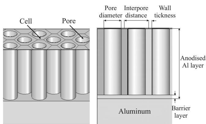
Fig. 5. Anodized aluminum structure
