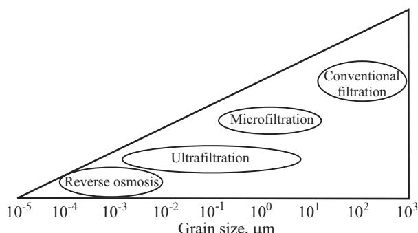
Fig. 4. Methods of filtration of particles depending on grain size
