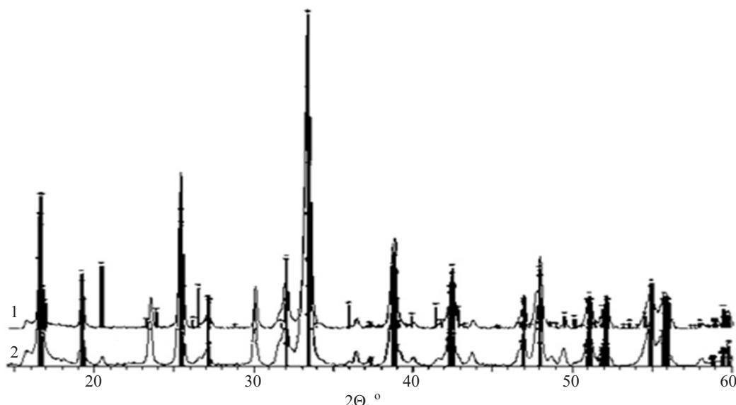
Fig. 3. X-ray diffraction of patterns of YAB nanopowders before (1) and after separation (2)
