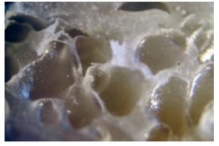
*Fig. 4. View of double-layered coatings structure containing blowing agent in amount 0.5 wt. %*
