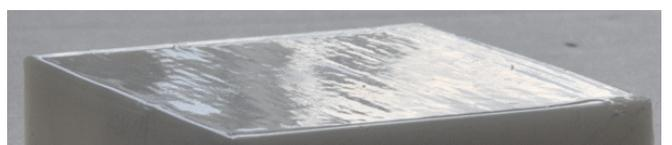
Fig. 11. Chemical treatment of ABS plastic samples using acetone
