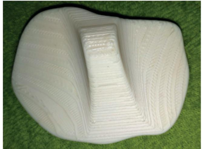
Fig. 4. Model made by FDM technique
